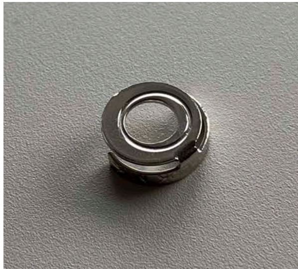
Misaligned Side Load VCR gasket
